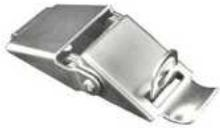
Catch with straight hook-Padlockable..Uses Strike Numbers SK-3700 and SK-3701.....Tension could be increased or decreased based on the distance between the holes in the Latch/Keeper
