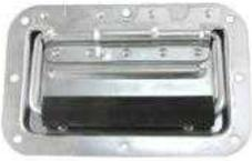
Handle-Recessed Dish-Return Spring Design Load is 200 lbs at 115 Degrees..Tested to 135 Lbs tension without significant failure to Plate or Bail. Temp. Range -52F to +150 F .. 358 Grams
