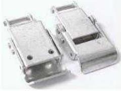
CA-3500 Family, downward Lever, Long Base...Uses Strike Number SK-3500 - Pull Test: 150 Lbs Min... at 370 Lbs..... 39 Gr.... VIBRATION & SALT SPRAY Reports per MIL-STD 202 are available. ...304SS for Stainless Parts.. Ultimate Strength: 600 Lbs.
