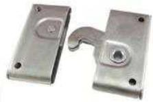
All parts are Zinc Plated except for cam (Brass). Ultimate Tensile load: 2,500 lbs....If Zinc Nickel plated, Finish meets the 500 Hours Salt Spray requirements per ASTM B117-11.. Test Reports are available...Total Weight: 337 Gr.
