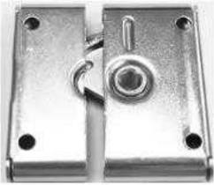
Panel Lock-Standard, Zinc plated. Part remains functional after 500 Hours Salt Spray. Total Weight: 238 Gr....Ultimate Tensile Load 1400 Lbs.. Ultimate Share Load 2000 Lbs....
