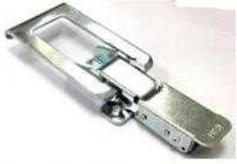
Adjustable Latch.....Tension could be increased or decreased based on the distance between the holes in the Latch/Keeper.... Tested at 2500 Lbs with no failure. Weight .85 Lb.
