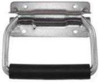
Same as HA-8000 except, Bail has an offset angle (overall Dim. is 4 5/32 Ref.)..Tested to 175 Lbs tension without significant failure to Plate or Bail.
