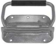
Handle, 90 Degree Stop, 302SS Spring, Neoprene Grip )...Temp Range for R. Grip is (-52 F to +150F). Plate: 6061 Caustic Dip and Alodine treated....Spring is DFARS Compliant, Spring is made and Handle is assembled in USA.
