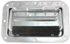
90 Degree Stop with return spring.. Design Load is 200 lbs at 115 Degrees...358 Grams Temp. Range -52F to +150 F ..Tested to 135 Lbs tension without significant failure to Plate or Bail.
