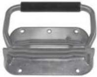
Same as HA-9450 EXCEPT, BAIL IS LARGER AND SPRING ENDS GO THROUGH TWO HOLES...Parts were tested to 4 KN (900 Lbs.) tension without any significant deformation to components. Approx. 225 Grams.
