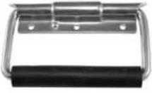
Handle with Return Spring, stops at 90 degrees...Weight is 245 Gr. ..Tested to 135 Lbs tension without significant failure to Plate or Bail.
