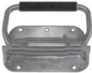
Refer to Chart.. 90 Degree Stop, Return Spring.....Parts were tested to 4 KN (900 Lbs.) tension without any significant deformation to components. Approx. 225 Grams. Hole Dia. is .199 and all Steel parts are Zinc plated (CZ). Aluminum Parts are 6061, T4 for Bail and T6 for Plate
