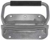
Handle, 90 Degree Stop, 302SS Spring, Neoprene Grip )...Temp Range for R. Grip is (-52 F to +150F). Plate: 6061-T4 Caustic Dip and Alodine treated....Spring is DFARS Compliant, Spring is made and Handle is assembled in USA. Parts were tested to 4 KN
