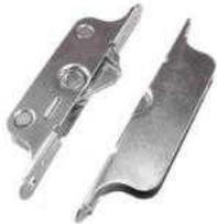
Zinc plated. Ultimate tensile load: 1400 Lb. Ultimate Shear Load: 2000 Lb..Latch Failure in wood before 600 Lbs...If Zinc Nickel plated, Finish meets the 500 Hours Salt Spray requirements per ASTM B117-11.. Test Reports are available...Total Weight: 230
