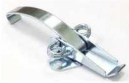
Long Blade...46 Gr...Clamping Force :75 Lbs - 160 Lbs.for Steel and 60-120 Lbs for Stainless, Average Ultimate Load: 400 for Steel and 380 for Stainless. Uses SK-4000 Strike.....Tension could be increased or decreased based on the distance between the ho
